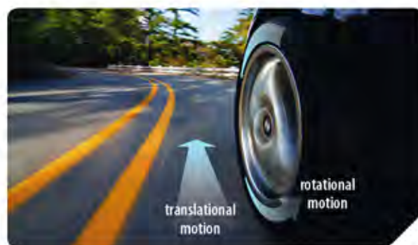
Fig. 5.4 Translational v. rotational motion
